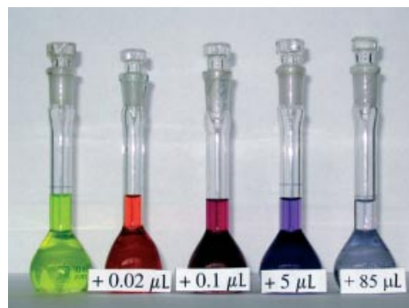
Figure 4. Color change of a 2.44 \cdot 10^{-5} M solution of 9 in \text{CH}_2\text{Cl}_2 by addition of \text{CF}_3\text{COOH} .
